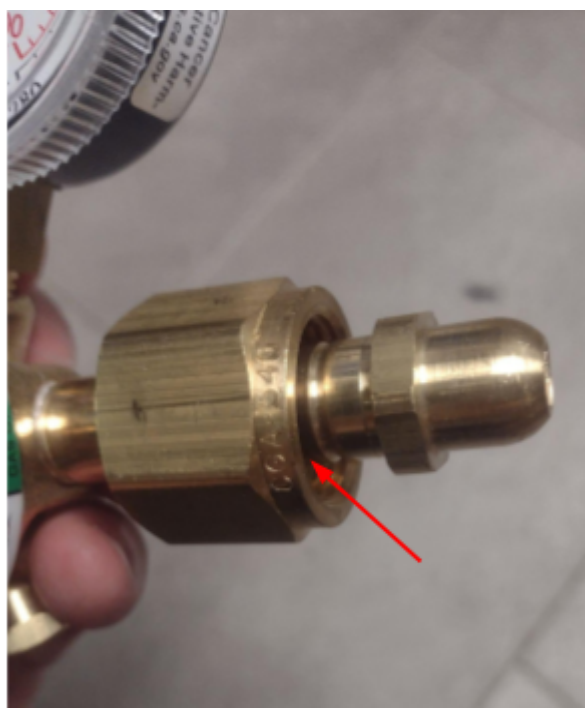
Note the CGA540 markings on the nut
