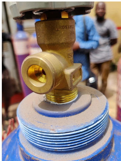
Figure 9 & 10: German valve examples with identifying markers
