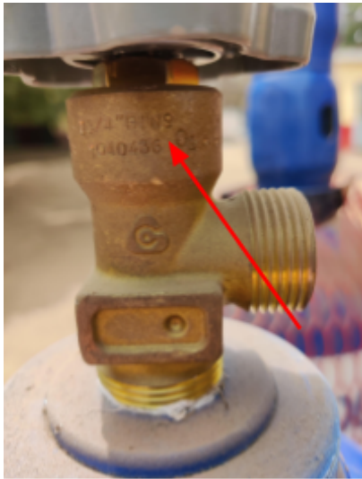
Figure 9 & 10: German valve examples with identifying markers
